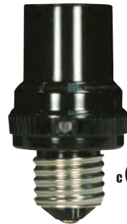
90-2604 Brown Medium to Medium Adapter E26 - E26 with Photocell, Overall Ext. 2" 150W-120V (incandescent), 60W-120V (fluorescent) - 11W-LED Suitable for Dry or Damp Location - CSSNP
