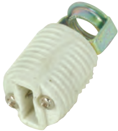
80-1582 Porcelain Socket Push-In Terminals 1/8 IP Hickey Inside Extrusion Double-Leg 1 1/2" H x 3/4" Dia. 500W-250V - 2Amp
