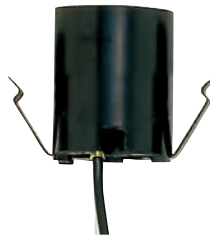
80-1645 Snap-In Socket for 3 1/4"-4" Holders 12" AWM B/W Leads 125°C Ht. 1 1/2" Dia. 1 1/4" 660W-250V
