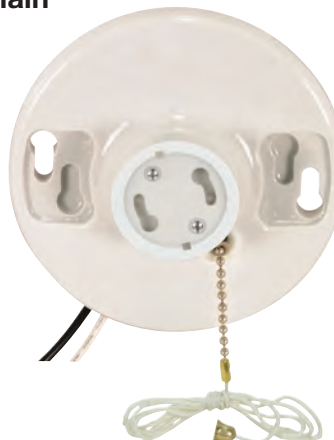
90-2582 Pull Chain White Porcelain GU24 On-Off Pull-Chain Ceiling Receptacle 6" AWM B/W Lead 4 3/8" Dia. 660W-250V
