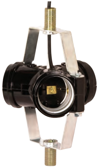
90-463 3 Light Cluster Socket 1 3/4" 1/8 IP Threaded Top Bracket w/ 5/8" Nipple 1 3/4" 1/8 IP Threaded Bottom Bracket w/ 5/8" Nipple 12" AWM B/W Leads 105°C 660W-250V
