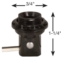
90-1556 1 1/4" w/Shoulder and Phenolic Ring 8" AWM B/W Leads 105°C 75W-125V Ring 1 1/8"
