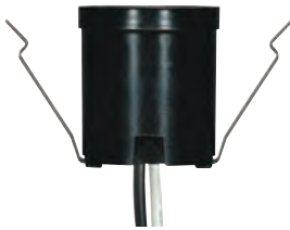
80-2299 Snap-In Socket w/Top Rim & for 3 1/4" - 4" Holders 9" AWM B/W Leads 105°C Ht. 1 1/2" Dia. 1 1/4" 660W-250V
