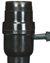
80-1107 3 Terminal (2 Circuit) Turn Knob 1/8 IP Cap w/Metal Bushing Less Set Screw 2 7/8" H x 1 1/4" Dia. 250W-250V
