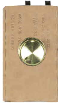
80-1293 Full Range Table Lamp Dimmer Switch Paper Housing 2" x 1 1/4" x 5/8" 12" AWM 105° C Black Leads Strip 1/2" w/Two Knobs: Black & Gold 60W-300W-120V
