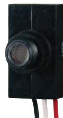
90-2633 Photoelectric Switch Plastic DOS Shell, Rated: 500W-120V 7.1A-850VA Ballast For Outdoor Use - HID 2" H x 1 1/8" W x 7/8" D
