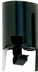
90-540 Snap-In Socket 6" AWM B/W Leads 105°C Ht. 1 1/2" Dia. 1 1/4" Bracket 1/4" Below 660W-250V
