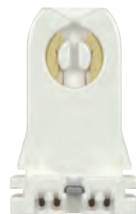
80-2022 Tall - T8 / T12 Lamps Turn-Type - G13 Base w/Screw & Nut Quickwire No. 18GA Designed For Electronic Ballasts 2 1/4" H x 1 1/4" W x 3/4" Dia. 660W-600V
