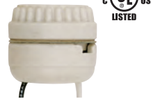
90-1111 Two Piece Medium Base Porcelain Sign Receptacle 8" AWM B/W Leads 105°C 1 1/2" H x 1 5/8" Dia. 80-2296 9" Leads 660W-250V
